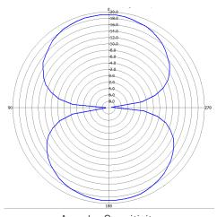
Angular Sensitivity (Relative Read Range vs. Orientation)
