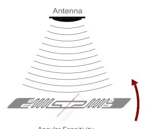
$\label{eq:Angular Sensitivity}$  Inlay is rotated in the x, y, plane about the z axis
